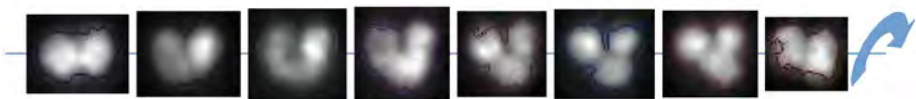
Fig. 2: Fluorescence stained nucleus of a white blood cell. Object boundaries (Contours) for feature measurement by Digital Image Analysis are drawn as circumference lines in the thumbnail images. A 180 degree rotation is recorded within a single transition of the cell trough the detection chamber of the chip.
